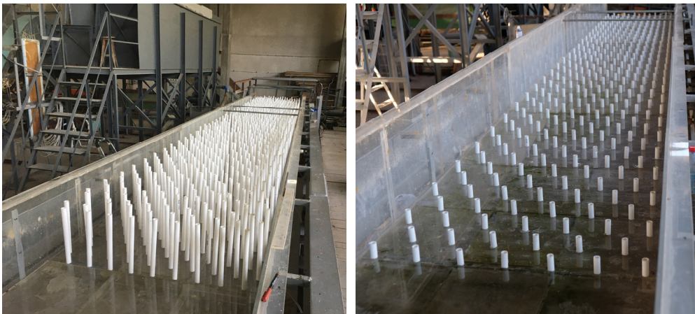
Figure 4.5. Placement of rigid vegetation stems for emergent and submerged cases
